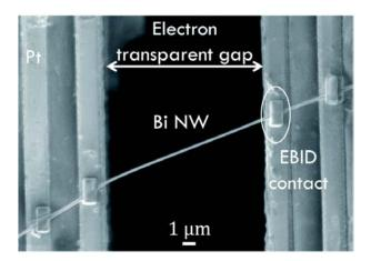
**Above**. Scanning electron microscopy image of a Bi nanowire placed on the thermoelectric nanowire characterisation platform.
